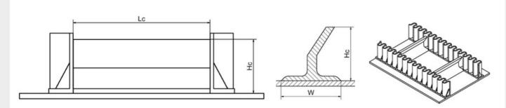
The right choice of type, dimensions and rubber compound ensures a suitable solution for any operating requirement and for any type of material. All cleats are designed with a flat base to ensure a uniform adhesion and to adapt to a reduced wrap diameter on pulleys.
