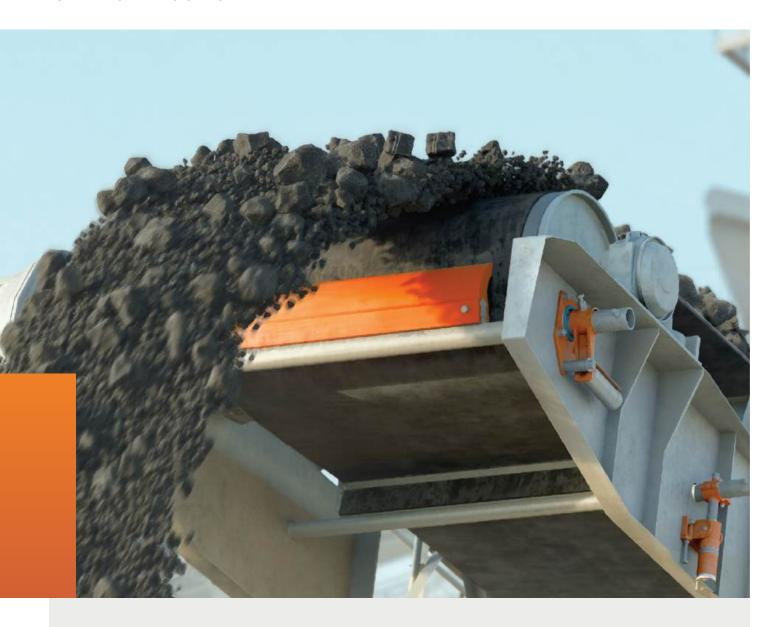
The primary cleaning system is the first cleaning element that removes most of the material adhered to the conveyor belt, leaving only a thin layer of fine grain.
